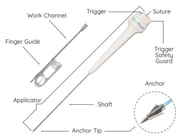
When the "exit" line is visual the anchor is within the Work Channel and no tissue trauma will occur. Once the line is covered by the port, the needle is exposed distally and tissue trauma is possible.
